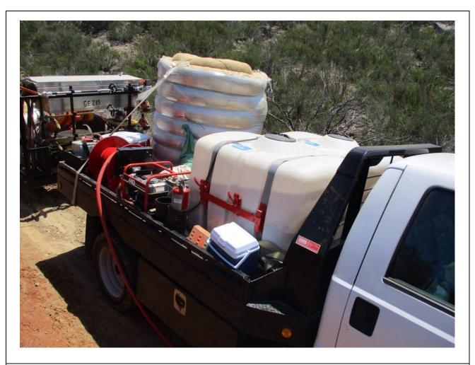
**Photo 4:** In addition to a 5 gallon backpack pump, round point shovel, Pulaski, and 2A10BC fire extinguisher, the vegetation clearing crew at Z571449 (TL6957) was equipped with 100 gallons of water with a pump and hose (as required for chipping) and a crew member was observed wetting down the area during chipping in accordance with the CFPPP fire prevention matrix (on CNF land).
